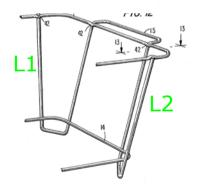
A wire chafing stand comprising a first rim of wire steel which forms a closed geometrical configuration circumscribing a first surface area, and having at least two wire legs with each wire leg having two upright sections interconnected to one another in a configuration forming a base support.... and further comprising a plurality of offsets located either in said upright sections of said wire legs or in said first rim for laterally displacing each wire leg relative to
